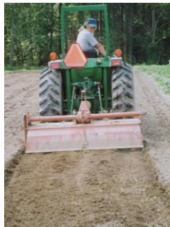
The rototiller is set to work just one inch deep, removing tiny weeds and incorporating cover crop seed.
