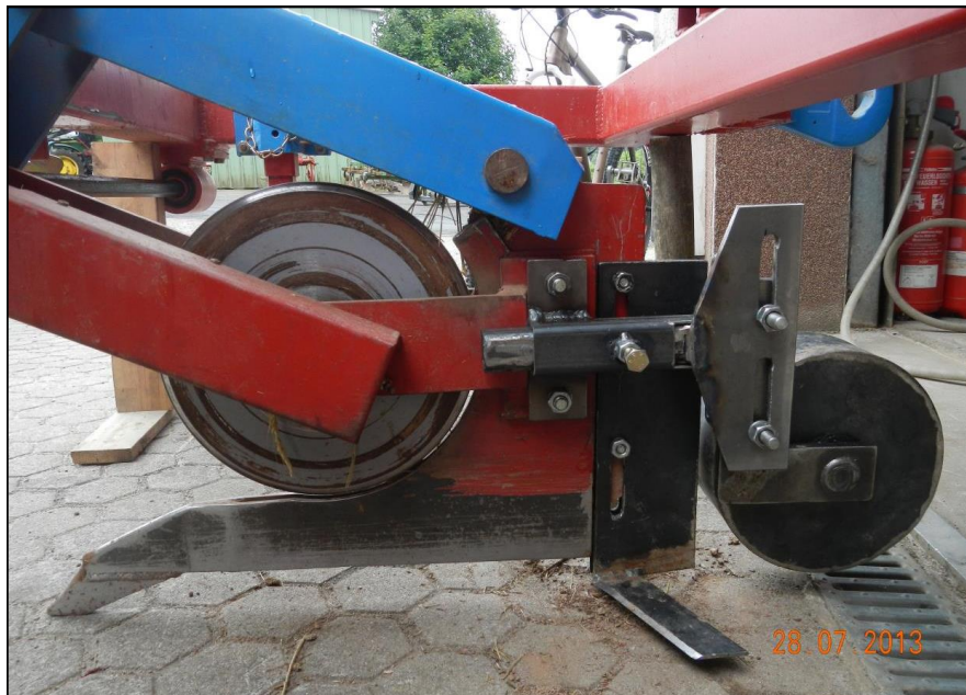
Mulch-Row-Cutter with wings as a sub-surface hoe / cultivator
