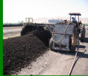
Compost: Modified Lubke method. Close-up of compost turner.
